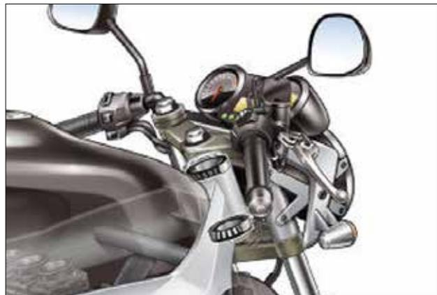
Position of the steering races in the steering column of a two-wheeler.
